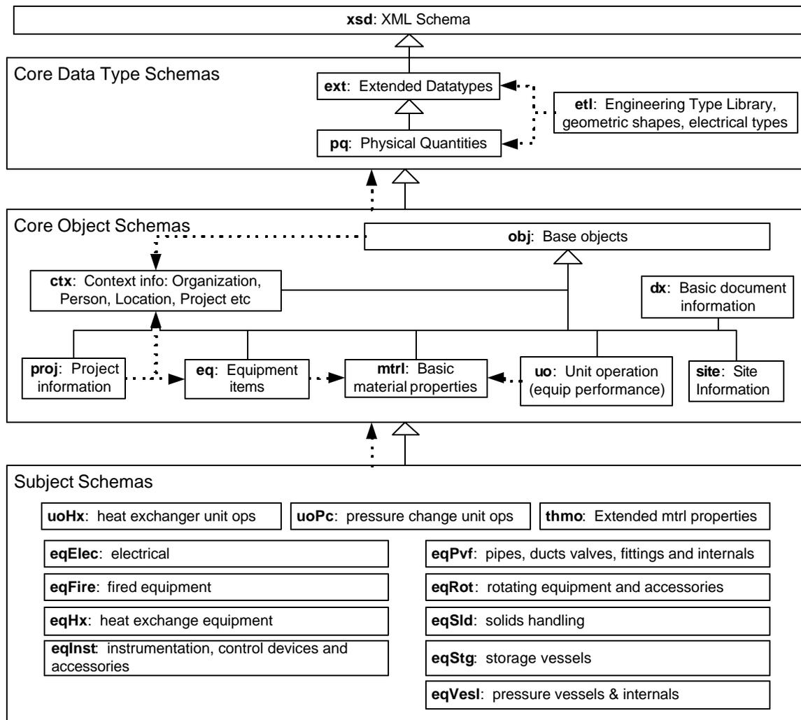
As can be seen from the above, the AEX project has approached a very large subject domain from an overall schema organization and architectural viewpoint, while creating detailed schemas for two equipment types – centrifugal pumps and shell and tube exchangers. As part of the scope definition, there are over 300 equipment types that may eventually be covered by the AEX effort to cover the broad range of equipment encountered in capital facilities.
