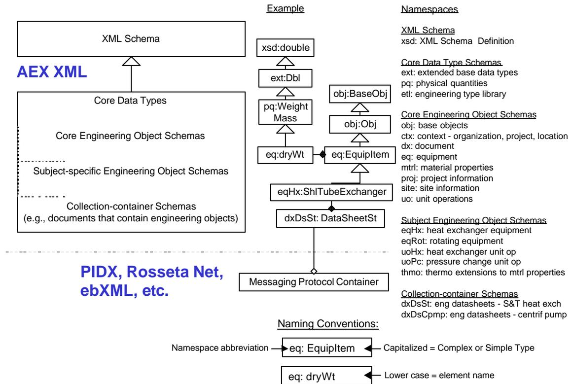
**Figure 1. Overview of AEX XML Schema Architecture**
